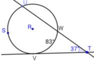
An angle formed by a secant and a tangent is One-half the difference of its intercepted arcs.
