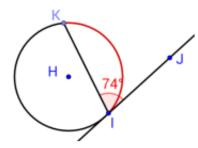
An angle formed by a chord and a tangent (vertex Is on the circle) is one-half its intercepted arc.
