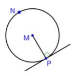
A radius is perpendicular to a tangent at the point of tangency.
