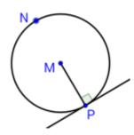
A radius is perpendicular to a tangent at the point of tangency.
