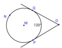
An angle formed by two tangents is one-half the difference of its intercepted arcs.
