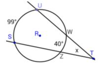
An angle formed by two secants is one-half the difference of its intercepted arcs.
